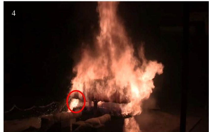
Figure 51 14:50 minutes: A large stream of sparks shoot out from the bottom of the NW end of the battery from its interior
