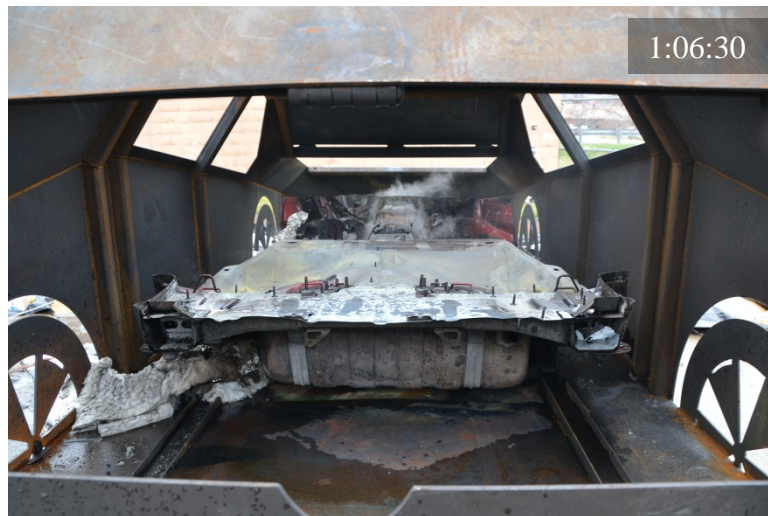
Figure 75 Test B1: suppression starts (top left); reignition and suppression (top right, bottom left); post suppression (bottom right)
