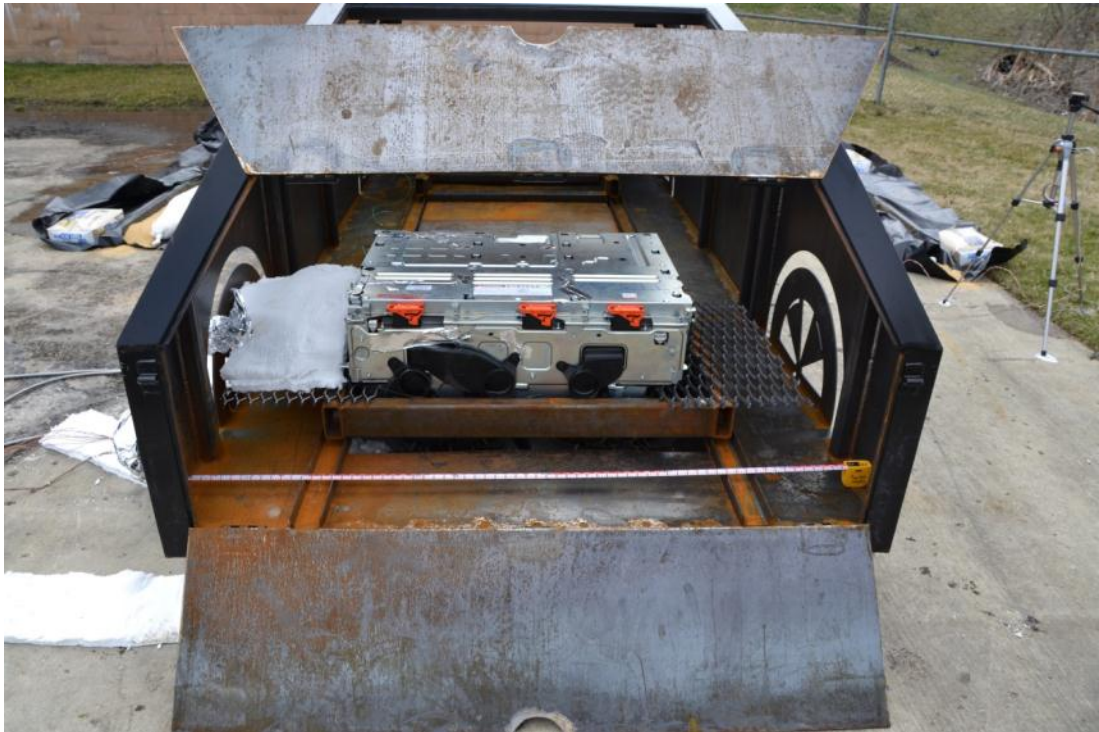
Figure 25 Carriage installed inside the VFT positioned above the four burners located in the rear test position
