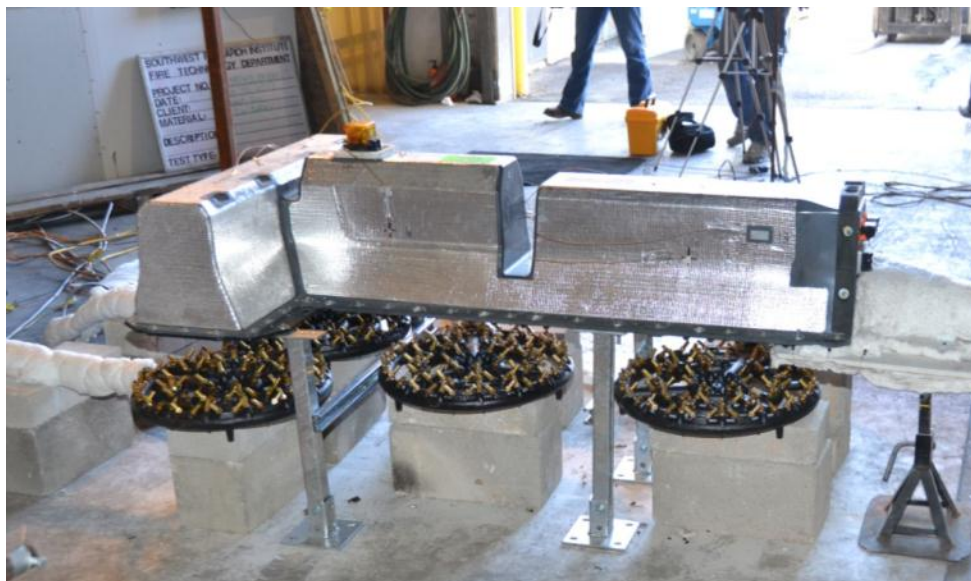
Figure 15 T-shaped burner arrangement comprised of four burners
