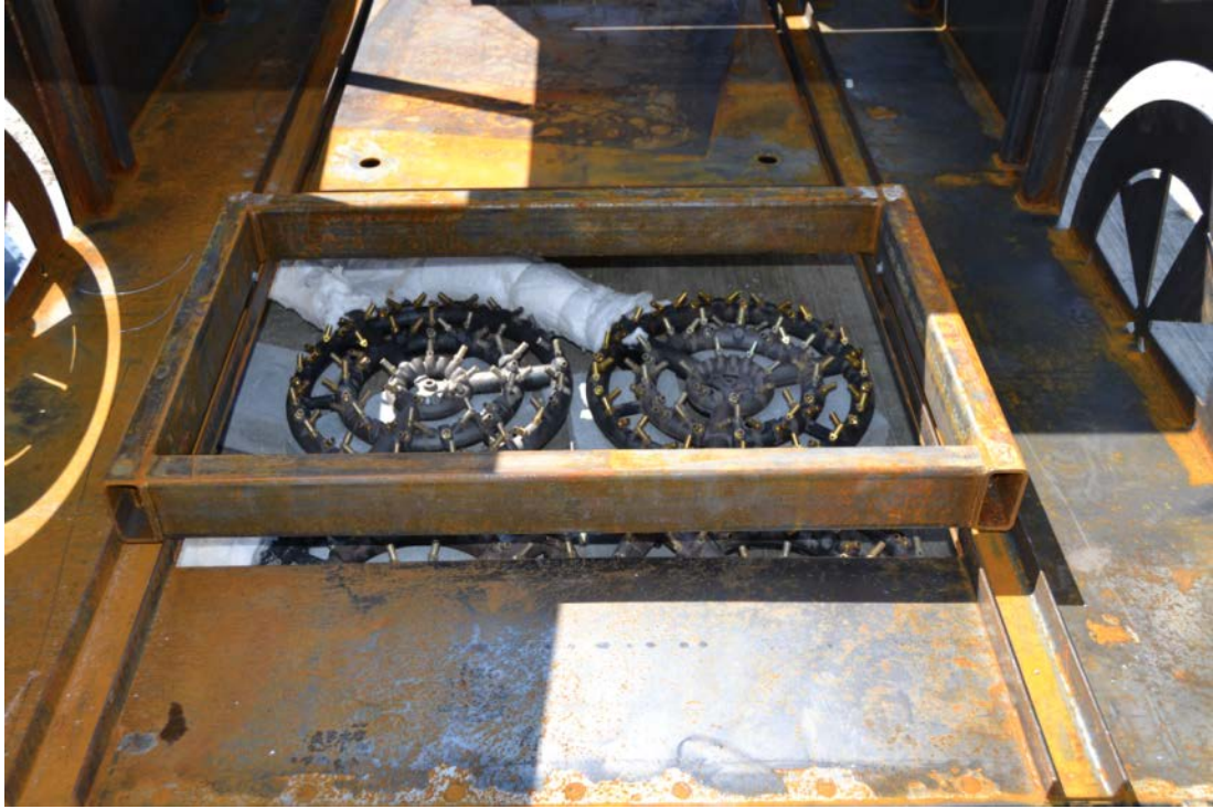
Figure 25 Carriage installed inside the VFT positioned above the four burners located in the rear test position
