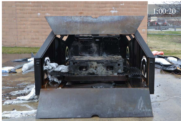
Figure 68 Test A3: Suppression starts (top left); reignition and suppression (top right, bottom left); post suppression (bottom right)
