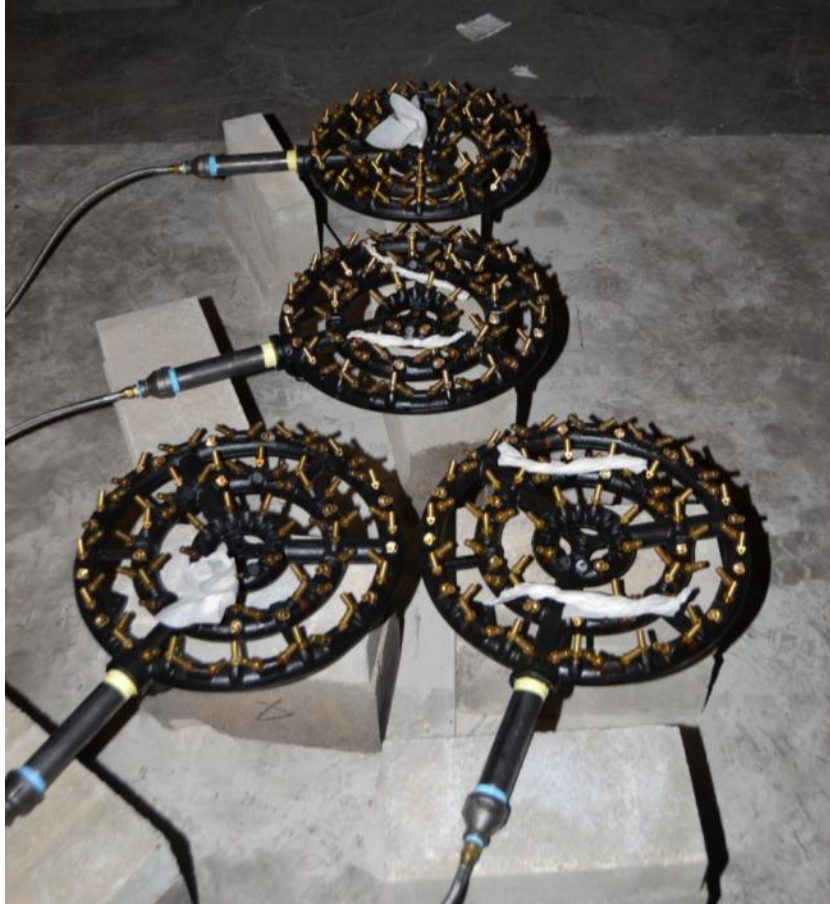
Figure 15 T-shaped burner arrangement comprised of four burners
