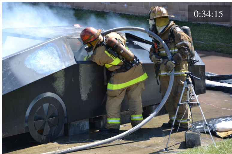
Figure 81 Test B2: suppression starts (top left); reignition and suppression (top right, bottom left); post suppression (bottom right)
