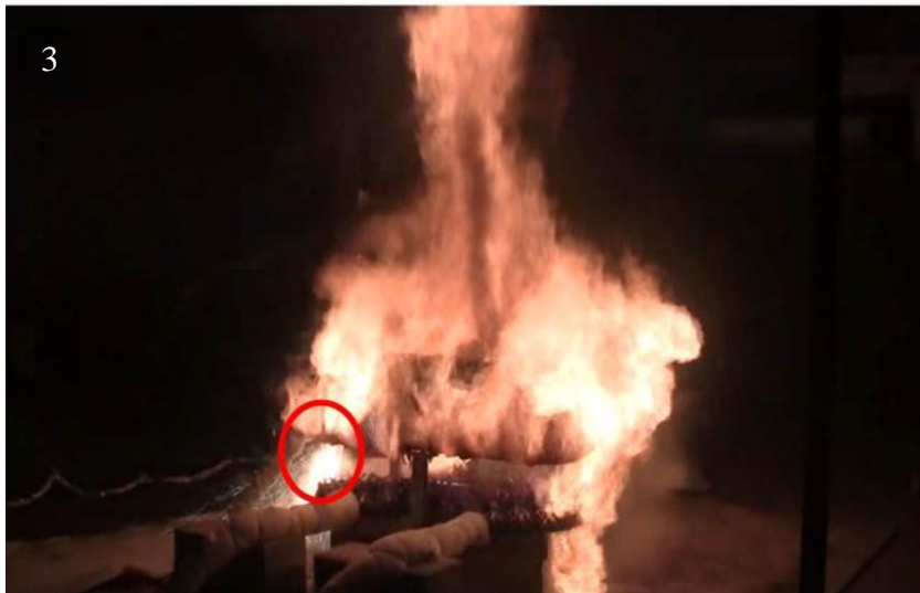
Figure 51 14:50 minutes: A large stream of sparks shoot out from the bottom of the NW end of the battery from its interior
