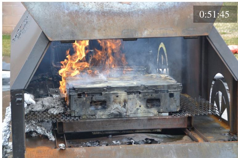
Figure 68 Test A3: Suppression starts (top left); reignition and suppression (top right, bottom left); post suppression (bottom right)
