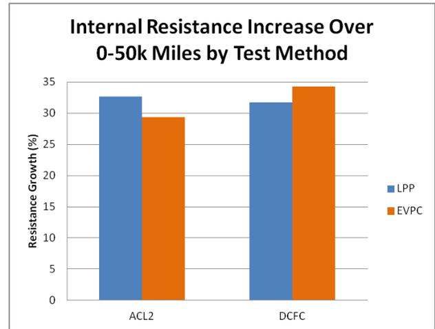
Figure 15. Battery internal resistance increase is shown between baseline and after 50,000 miles, as calculated using results from the low peak power and electric vehicle power characterization tests.
