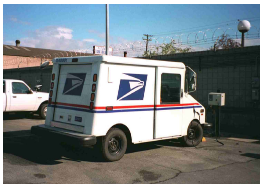
Figure 16. USPS light-duty electric delivery vehicle being charged at SCE.
