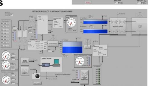
Low Pressure Storage/ PDC Compressor Displa
