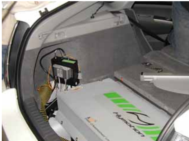
Figure 3. V2Green data logger (black box with cables) being installed inside the left rear of a Hymotion Prius PHEV conversion. The data logger and cellular modem (silver box in front of the V2Green module) is located up and to the left of the Hymotion/A123Systems PHEV battery.
