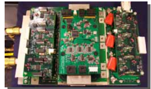
6 kW, 3-phase dc-dc converter
