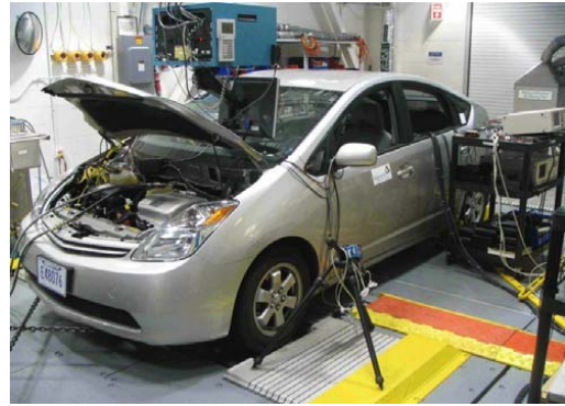
Figure 4. Hymotion Prius PHEV during chassis dynamometer testing.
