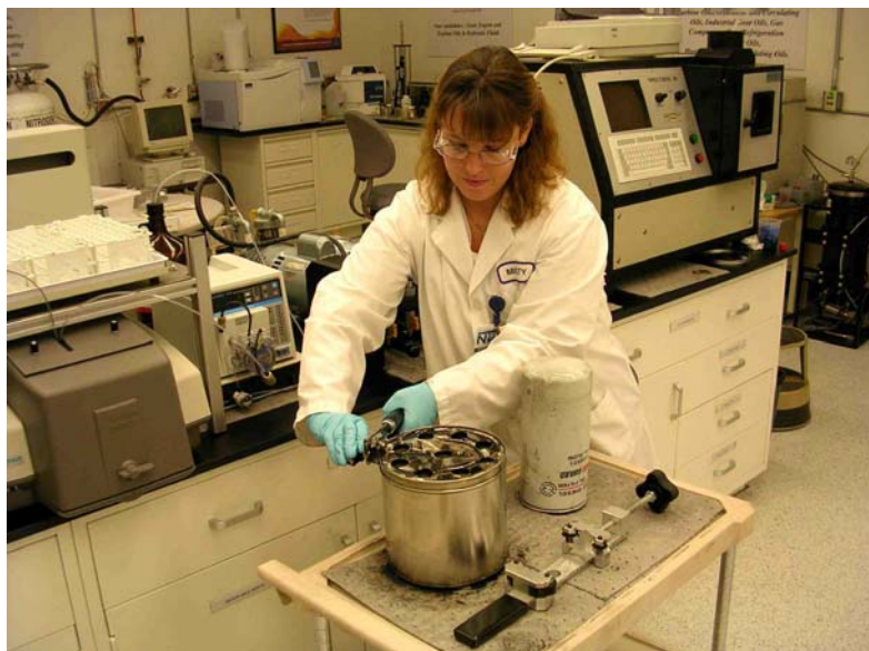
Figure 8. Removing the metal casing from the bypass filter (using second cutter).
