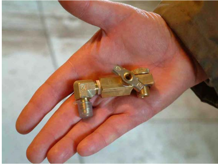
Figure 14. puraDYN orifice assembly with oil analysis sampling valve.
