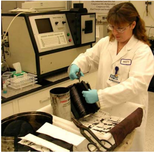
Figure 9. Filter media being dissected.
