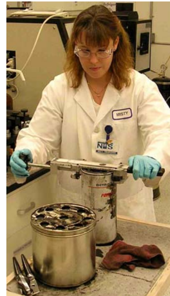
Figure 7. Removing the metal casing from the full-flow filter (using first cutter)
