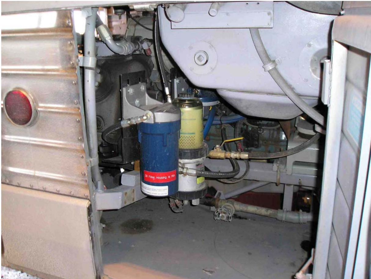
Figure 13. RGS bypass filter installation in the passenger side engine compartment.
