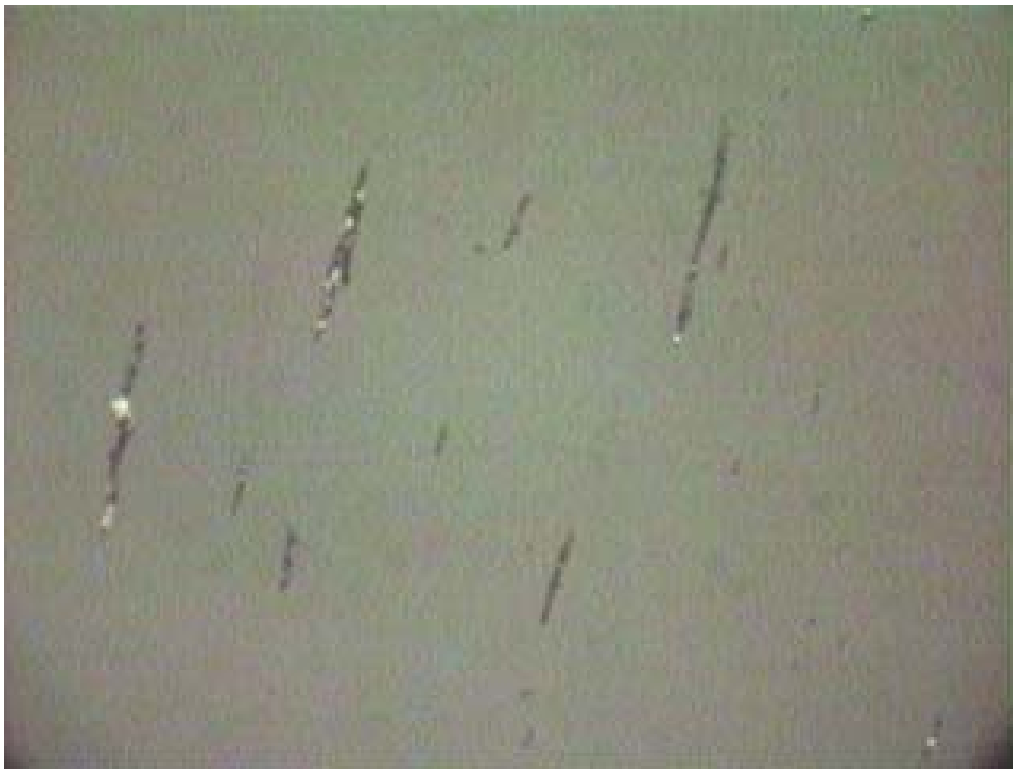
Figure 8. Picture (250x) of the ferrogram test for the sample taken March 4, 2004 from bus 73450.
