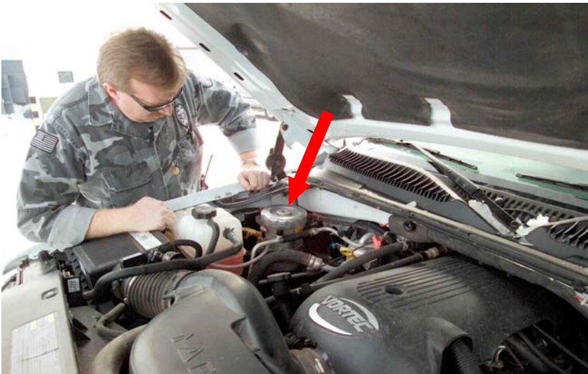
Figure 12. INL personnel viewing the location of the oil bypass filter installation in the engine compartment of an INL Chevrolet Tahoe.
