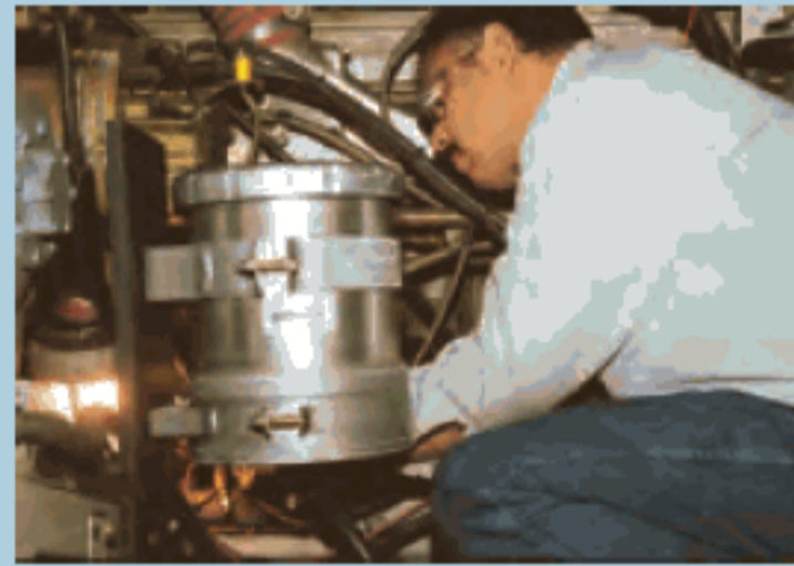
puraDYNE system in bus engine bay
