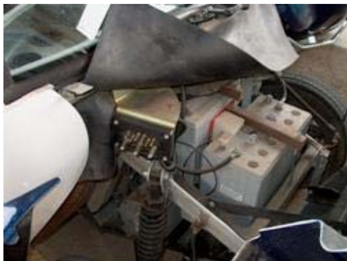
Figure 21. GEM fast charge inlet installed under the front hood.
