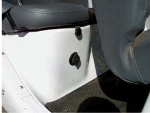
Figure 18. 2002 GEM 4-Passenger 120 V inlet located below the rear passenger side seat.
