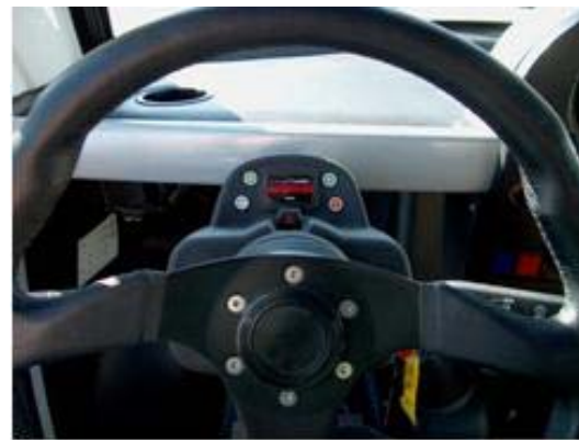
Figures 14A-B. Dynasty NEV SOC gauge, directional signals, high-beam indicator, charging indicator, and emergency flashers.
