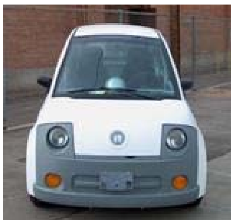
Figures 22A-B. Dynasty front fast charge inlet installed behind the license plate.
