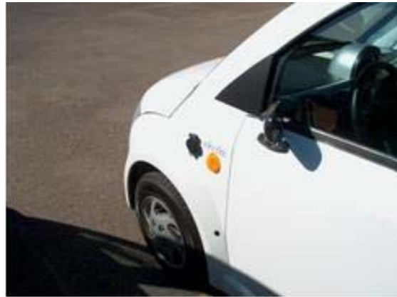
Figures 19A-B. Dynasty "It" 120 V inlet located on the driver's side front quarter panel.
