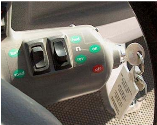
Figures 16A-B. GEM—turf /road selection and forward/reverse selection.
