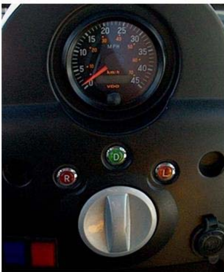
Figures 15A-B. Dynasty NEV center dash displaying the speedometer, odometer, gear selection, and heater/blower controls.
