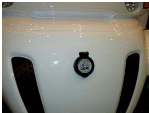
Figure 17. 2003 GEM—120 V inlet located in front hood under the GEM emblem.
