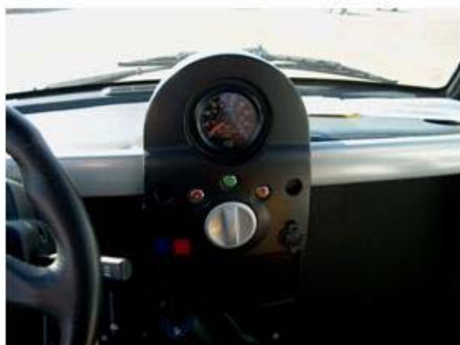
Figures 15A-B. Dynasty NEV center dash displaying the speedometer, odometer, gear selection, and heater/blower controls.
