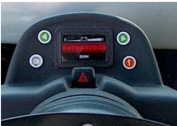
Figures 14A-B. Dynasty NEV SOC gauge, directional signals, high-beam indicator, charging indicator, and emergency flashers.
