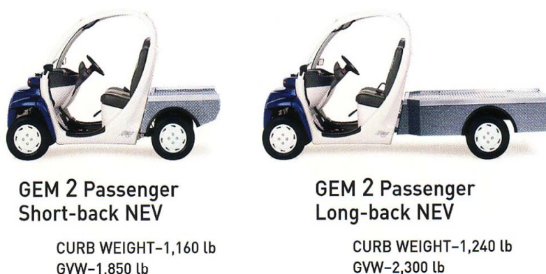
Figure 9. Typical payloads for NEV cargo haulers are up to 1,000 pounds.
