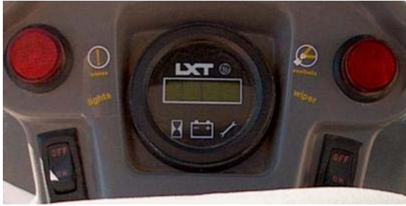
Figures 13A-B. GEM NEV dash with turn signal indicators, and an all-in-one digital display for speedometer, odometer, and battery SOC.
