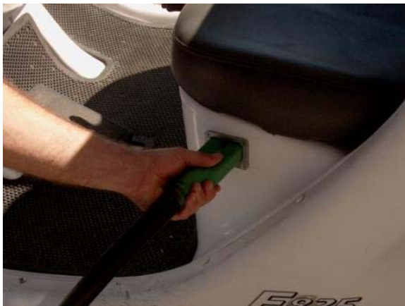
Figures 20A-B. GEM fast charge inlet installed on side of front seat support.
