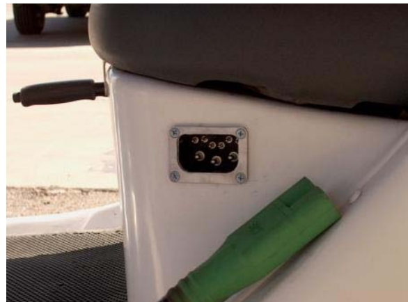
Figures 20A-B. GEM fast charge inlet installed on side of front seat support.
