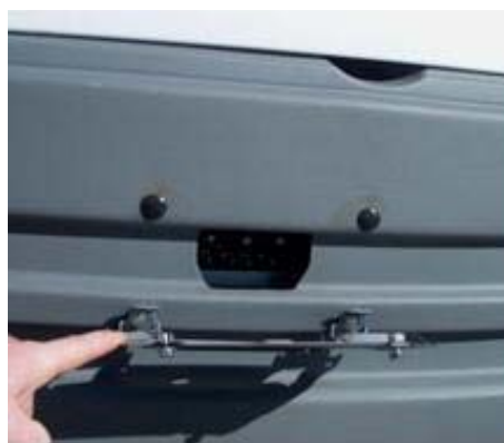
Figures 22A-B. Dynasty front fast charge inlet installed behind the license plate.
