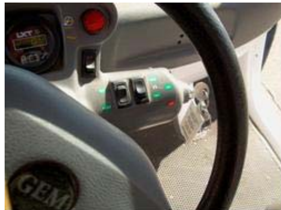
Figures 16A-B. GEM—turf /road selection and forward/reverse selection.
