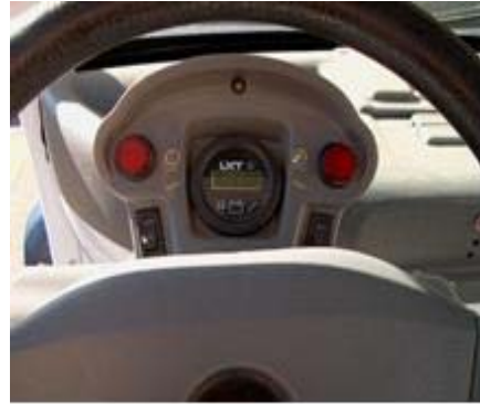
Figures 13A-B. GEM NEV dash with turn signal indicators, and an all-in-one digital display for speedometer, odometer, and battery SOC.
