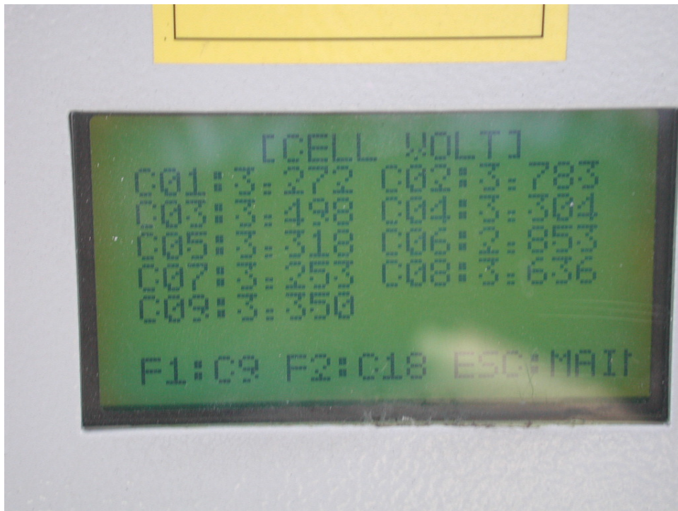
Figure A-4. Cell voltage display for cells 1 – 9.
