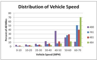
Data logged from diagnostic port using messages defined in SAE J1939 standard.
