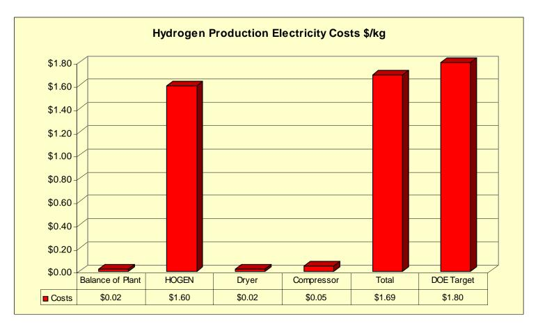
DOE 2005 Electricity Target (\$1.80) for a refueling station producing 250 kg/day. APS Hydrogen Production Electricity Cost based on APS published commercial/industry rate of \$0.02/kWh for 5 MW & larger.
