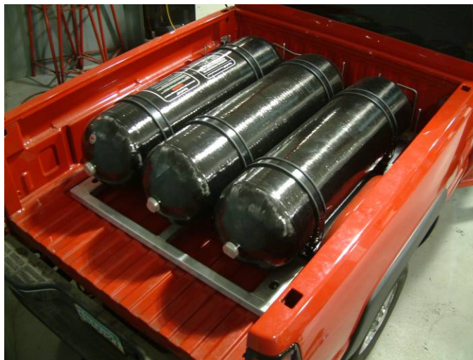
Figure 3-4. Silverado hydrogen internal combustion engine truck hydrogen storage.
