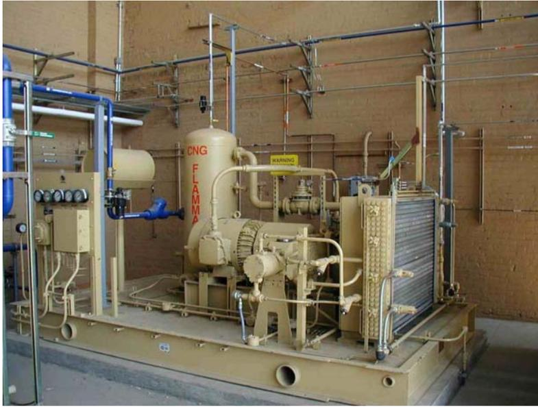
Figure 3.2. Gemini - main CNG compressor.
