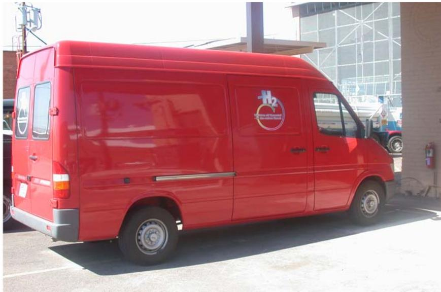
Figure 5. Mercedes Sprinter hydrogen-fueled van.
