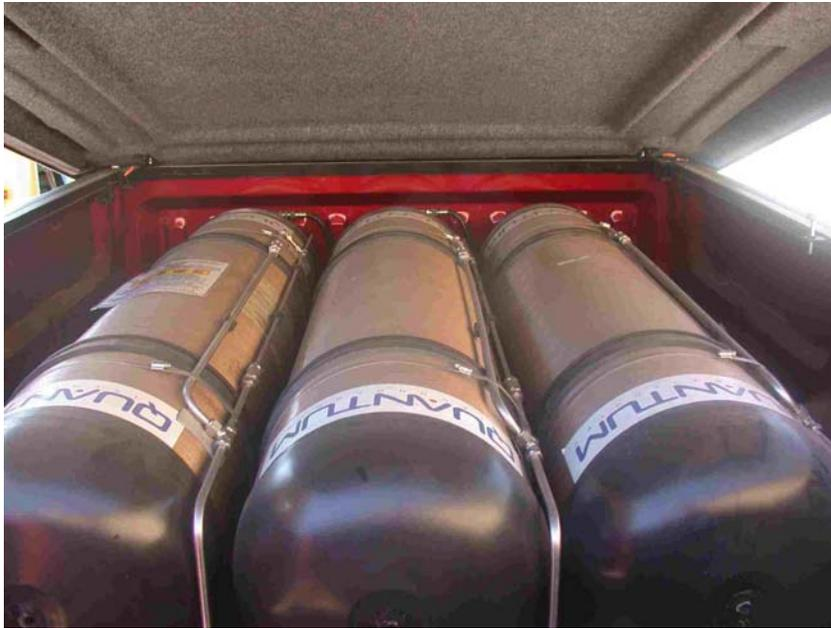
Figure 3. Quantum hydrogen fuel tanks.
