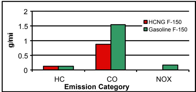
Figure 4. HCNG F-150 versus gasoline-fueled F-150.
