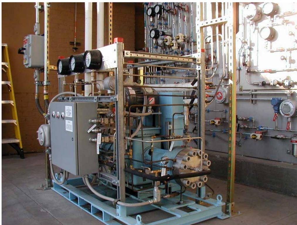
Figure 2.4. Pdc Machines, Inc. diaphragm hydrogen compressor.
