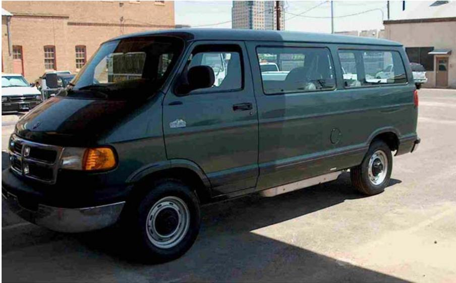
Figure 1. CNG- and HCNG-fueled Dodge Ram Wagon Van.
