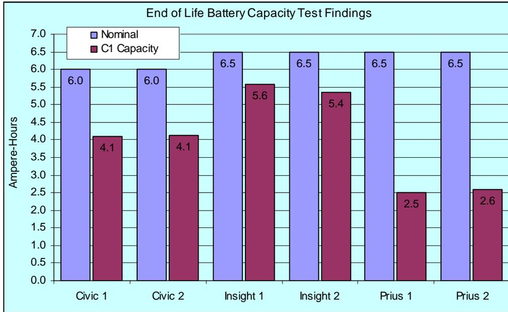
Figure 4. End-of-Life HEV battery capacity test findings.
