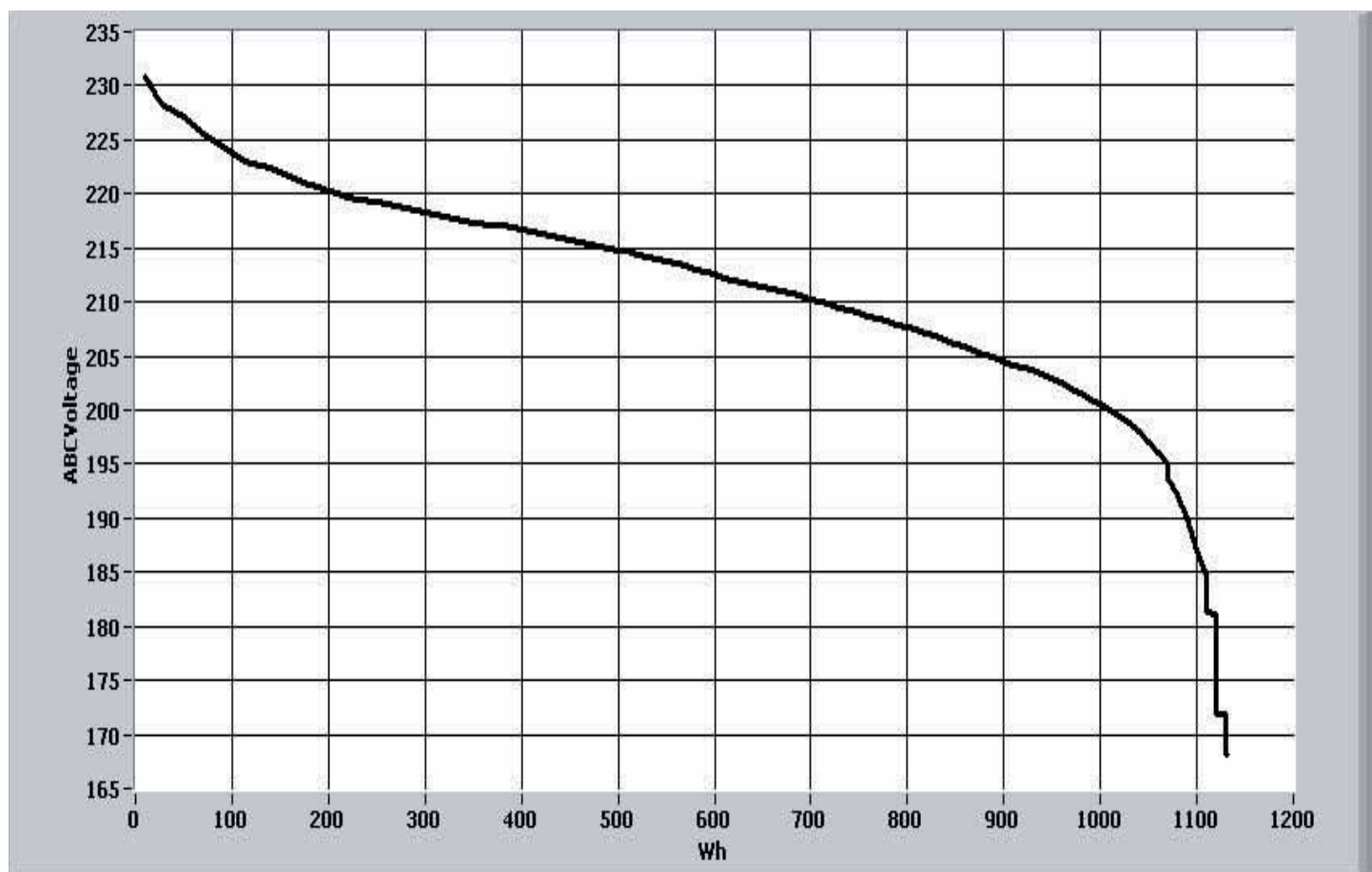
Figure 1 Voltage vs. Energy Discharged
