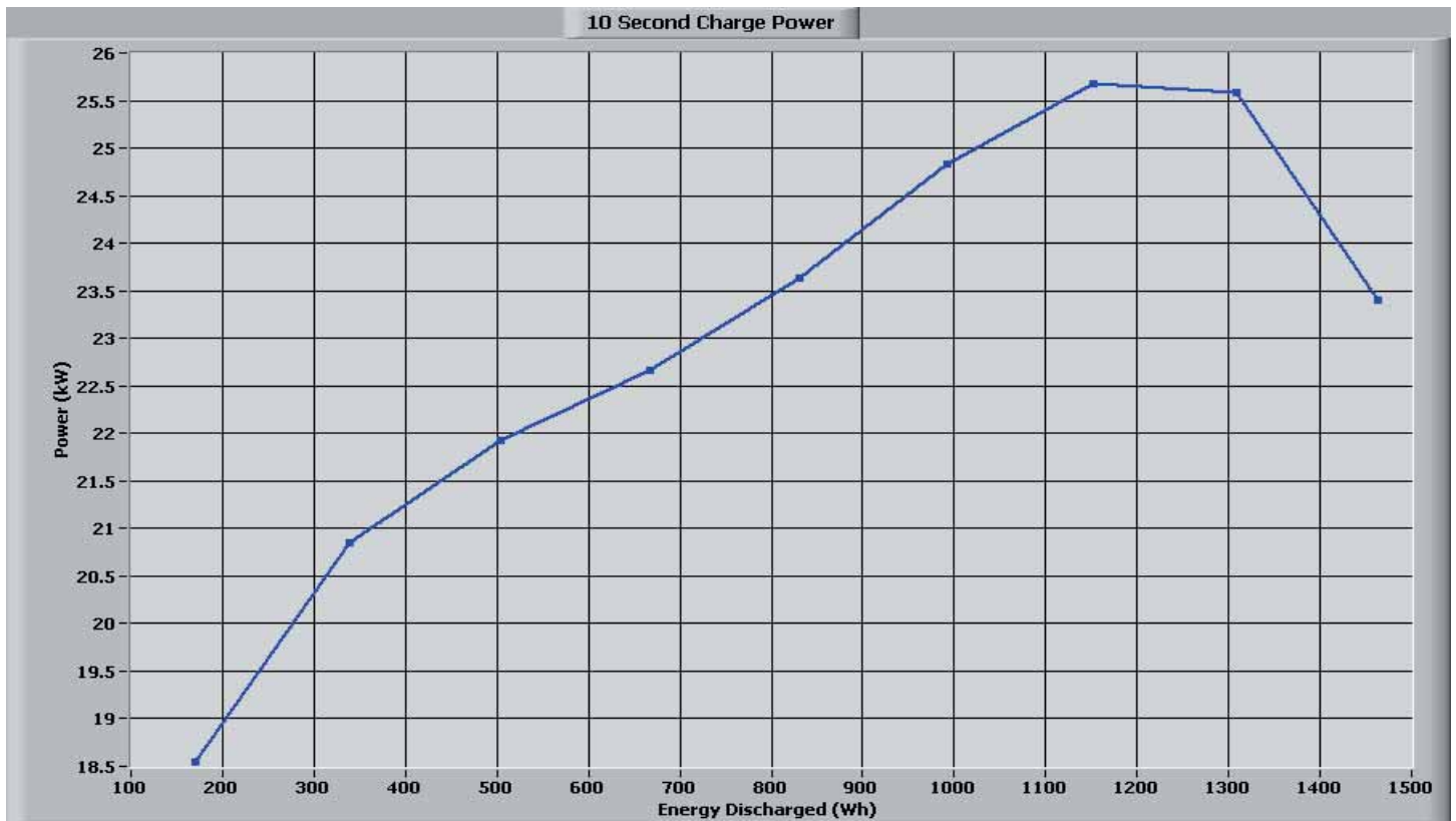
Figure 3 Charge Pulse Power vs. Energy Discharged
