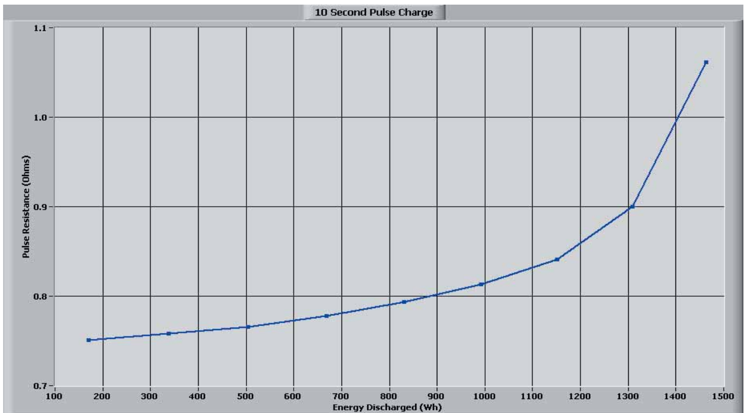
Figure 2 Charge Pulse Resistance vs. Energy Discharged
