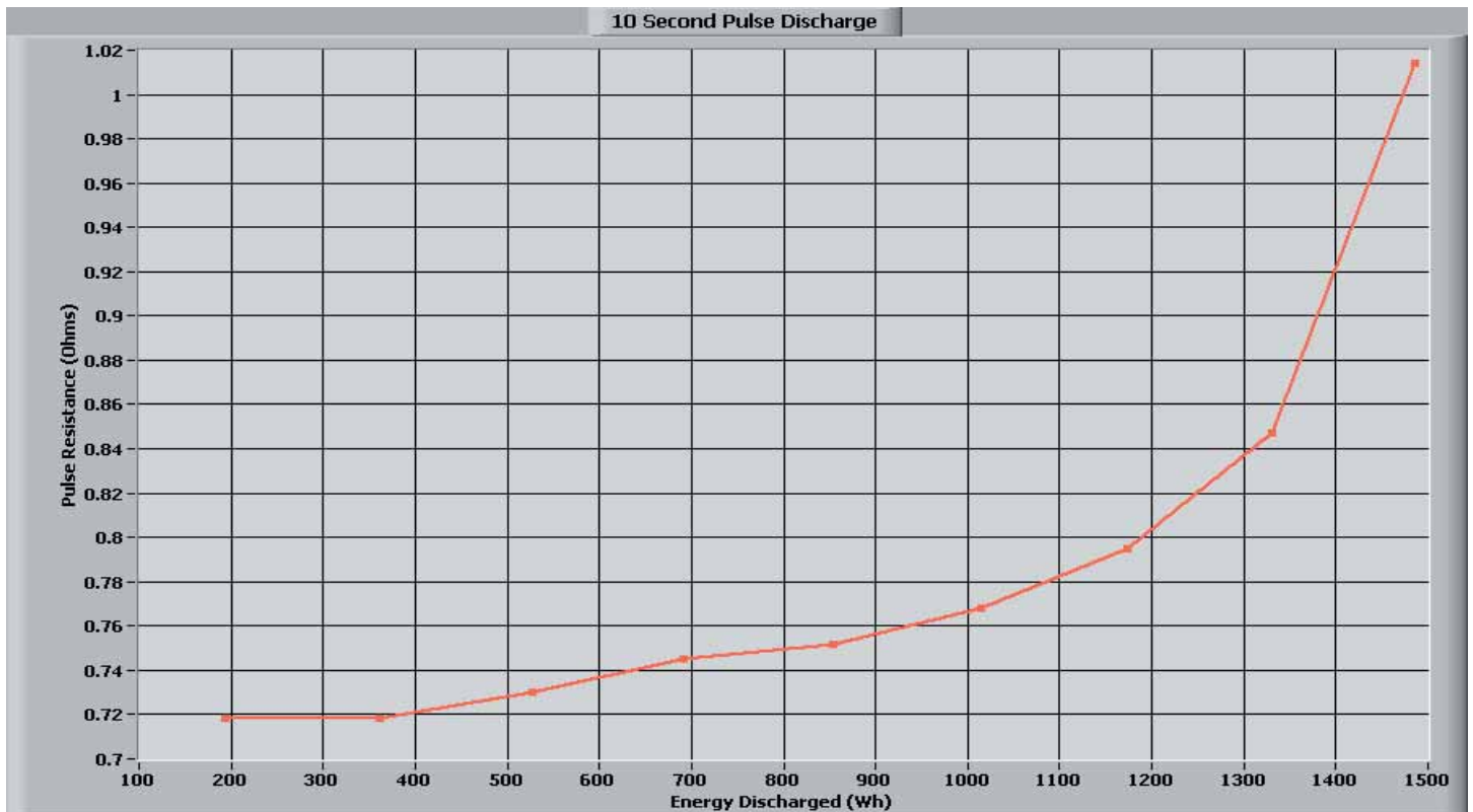
Figure 4 Discharge Pulse Resistance vs. Energy Discharged
