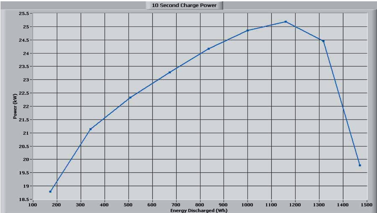
Figure 3 Charge Pulse Power vs. Energy Discharged
