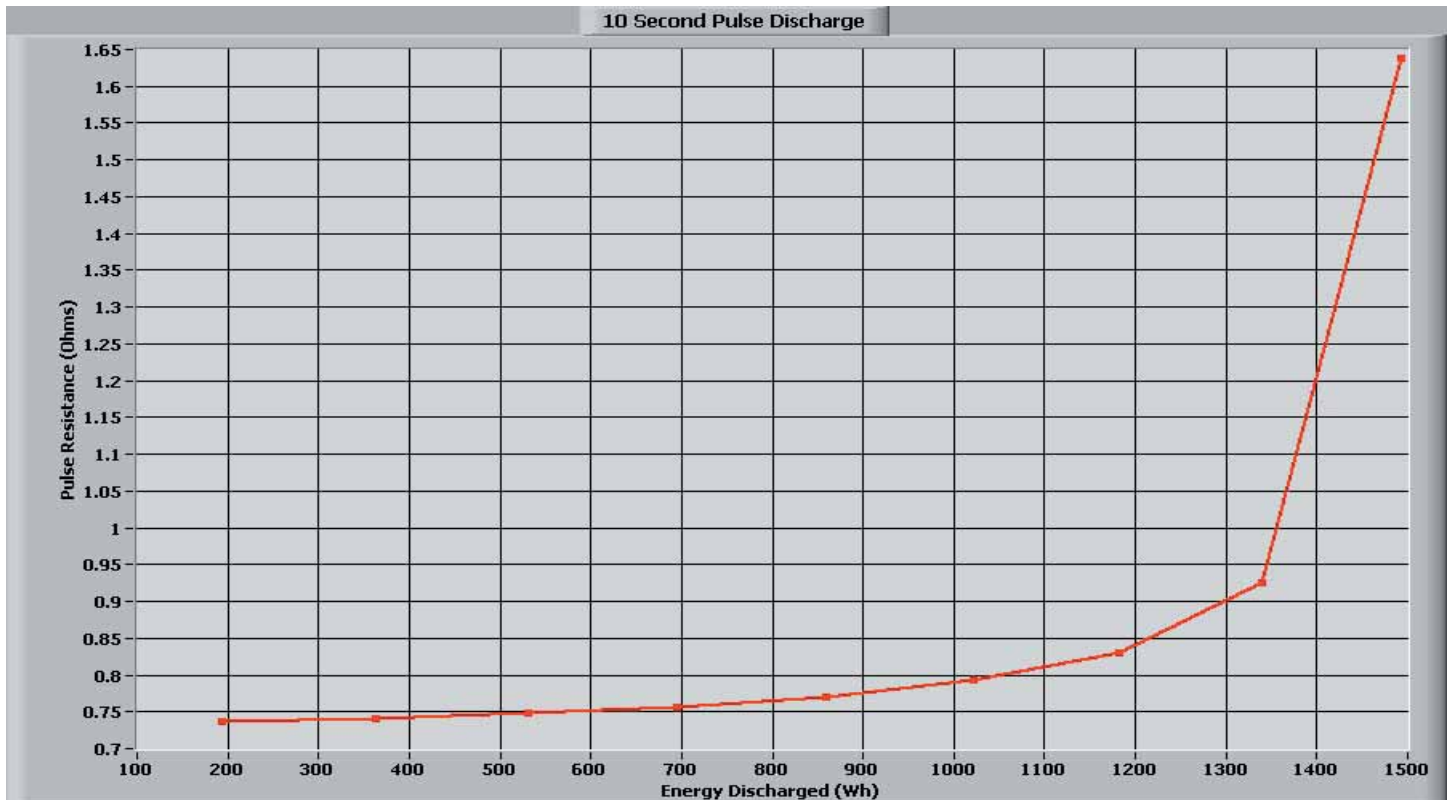
Figure 4 Discharge Pulse Resistance vs. Energy Discharged
