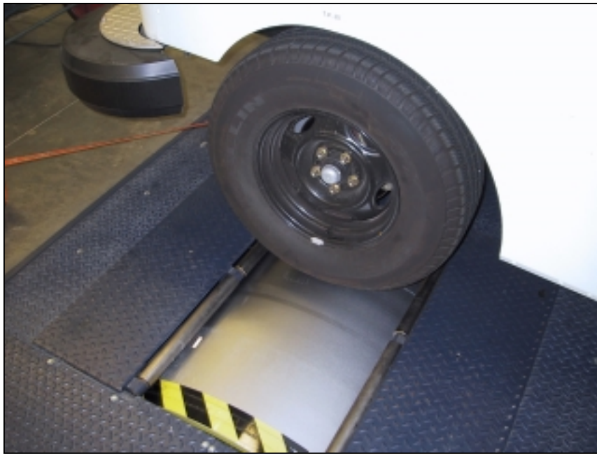
Figure 1 – 48-inch Roller of an AVL/Real Time Instrument's Electric Dynamometer
