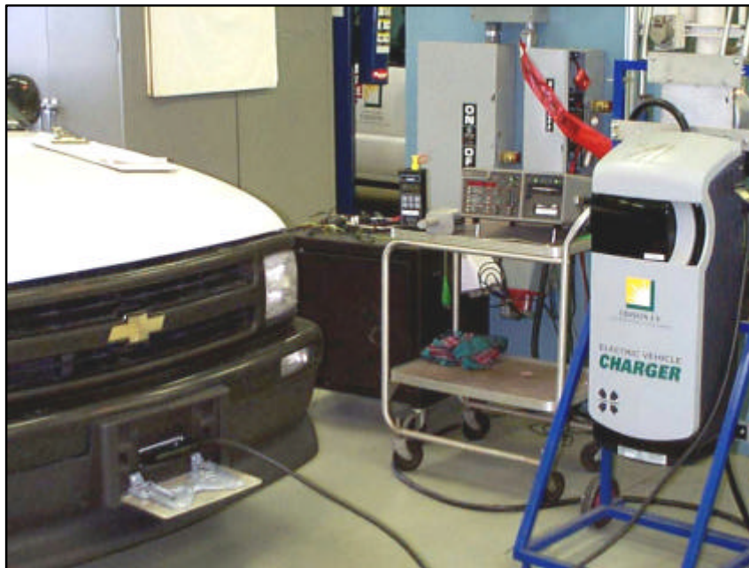
Figure 4-4. Charger testing with off-board 6.6 kW inductive charger.
