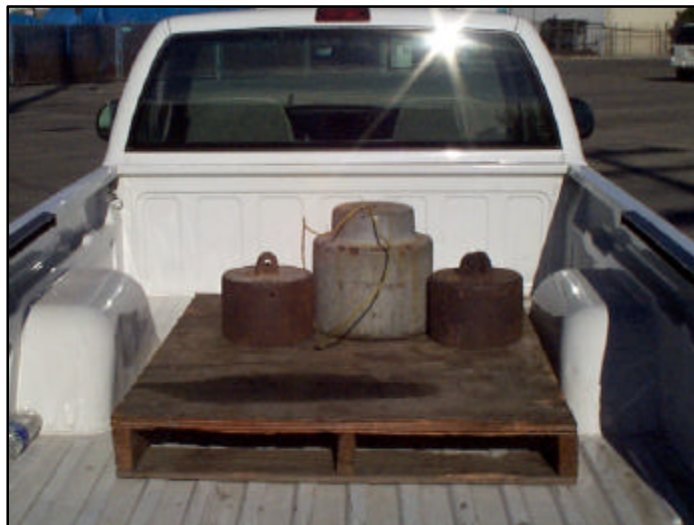
Figure 4-2. S-10 bed loaded with 550 lb.
