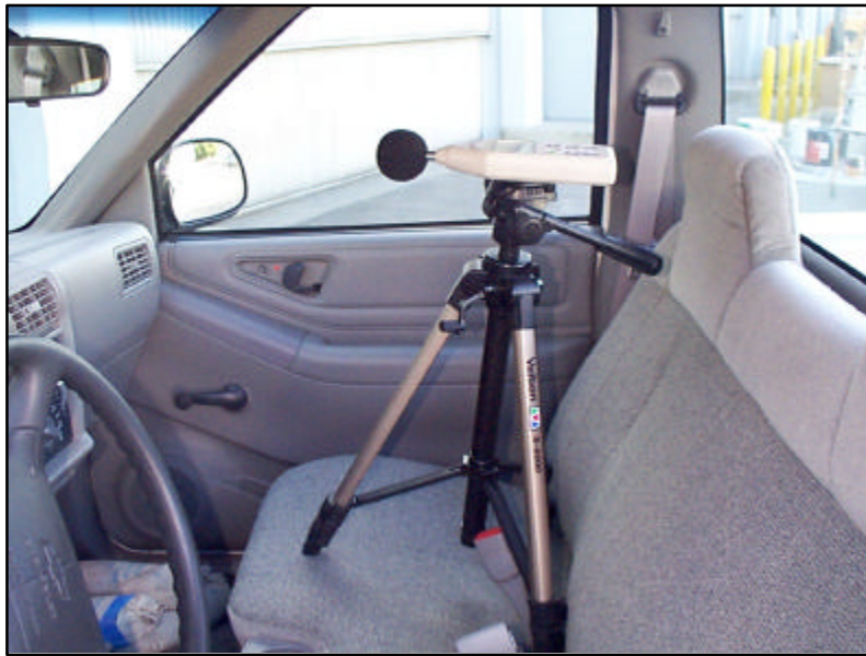
Figure 4-6. Sound level meter test setup.
