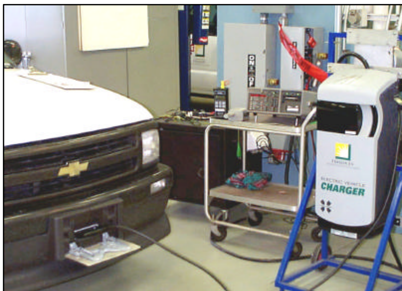
Figure 5-4. Charger testing with BMI Power profiler.
