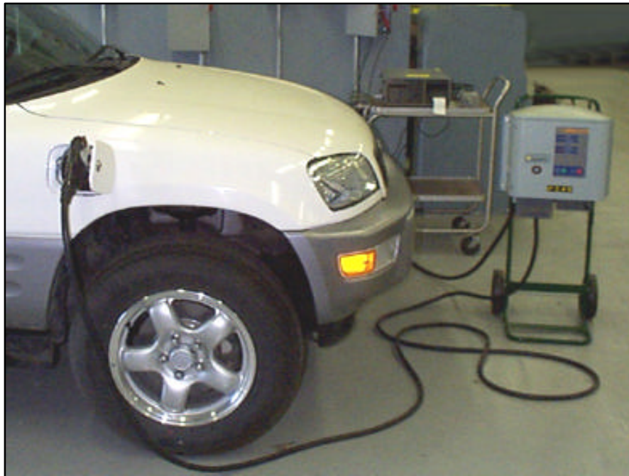
Figure 5-5. Charger testing with ICS-200 unit.
