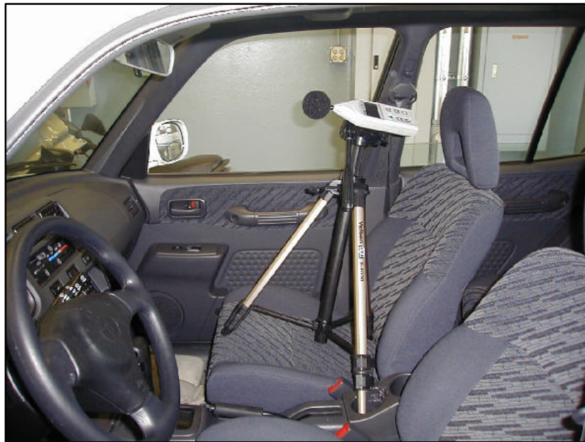
Figure 5-6. Sound level meter test setup.
