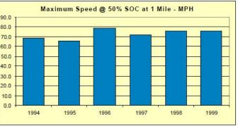
average maximum-speed test results shows a slight upward trend, especially when comparing the 1994 and 1995 averages to the 1996 through 1999 averages. Both the NiMH EV1 and lead-acid EV1 averaged 80 mph.
