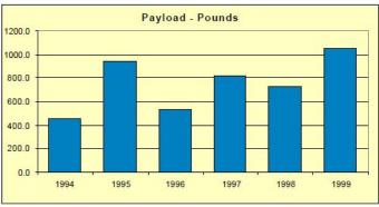
payload of 825 pounds. A single vehicle, the Baker pickup and its 1,719- pound payload, drove the payload average for the 1995 vehicles, while the other two 1995 test vehicles had an average payload of 546 pounds. The two 1996 test vehicles had an average payload of 533 pounds. One of these, the EV1, has a payload of 440 pounds. However, the EV1 is a sports coupe that clearly is not intended as a utility work vehicle with its light payload.
