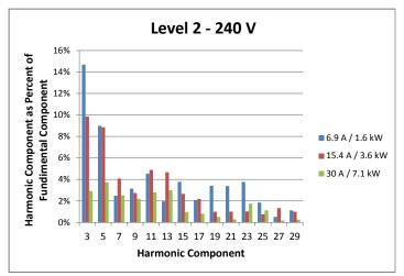
The harmonic components for three different charge rates are displayed in the charts above for both the Level 1 and Level 2 tests. For each test, the minimum charge rate (blue), maximum charge rate (green), and a charge rate between the minimum and maximum (red) were selected. In all cases, either the third or fifth harmonic is the dominant harmonic component.
