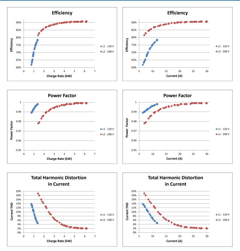
As the vehicle charge rate decreases, efficiency decreases, power factor decreases, and total harmonic distortion increases. The decrease in power factor is negligible, but the decrease in efficiency and increase in total harmonic distortion is not negligible and should be avoided when possible.
