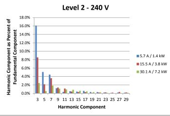
The harmonic components for three different charge rates are displayed in the charts above for both the Level 1 and Level 2 tests. For each test, the minimum charge rate (blue), maximum charge rate (green), and a charge rate between the minimum and maximum (red) were selected. In all cases, the third harmonic is the dominant harmonic component.
