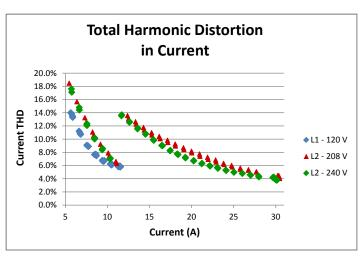
As the vehicle charge rate decreases, efficiency decreases, power factor decreases, and total harmonic distortion increases. For Level 2 charging, there is a step change in efficiency, power factor and total harmonic distortion at 13 amps or 3 kW..
