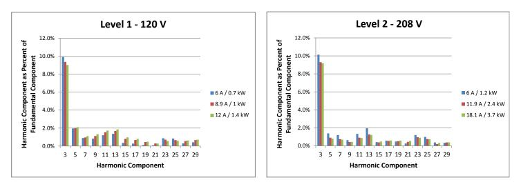
The harmonic components for three different charge rates are displayed in the charts above for both the Level 1 and Level 2 tests. For each test, the minimum charge rate (blue), maximum charge rate (green), and a charge rate between the minimum and maximum (red) were selected. In all cases, the third harmonic is the dominant harmonic component.
