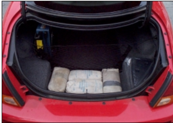
Figure 4-2. Trunk loaded with 100 lb.
