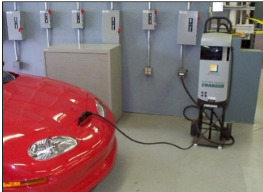
Figure 4-7. Charger testing with off-board 6.6 kW inductive charger.
