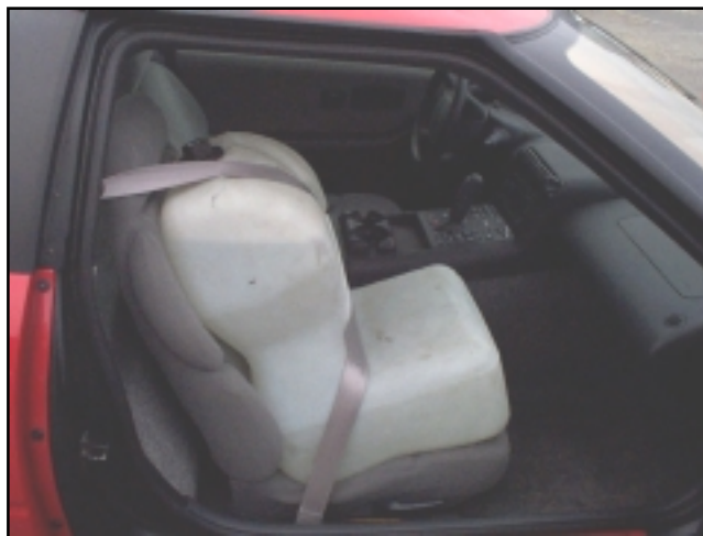
Figure 4-1. Passenger's seat loaded with 162 lb.
