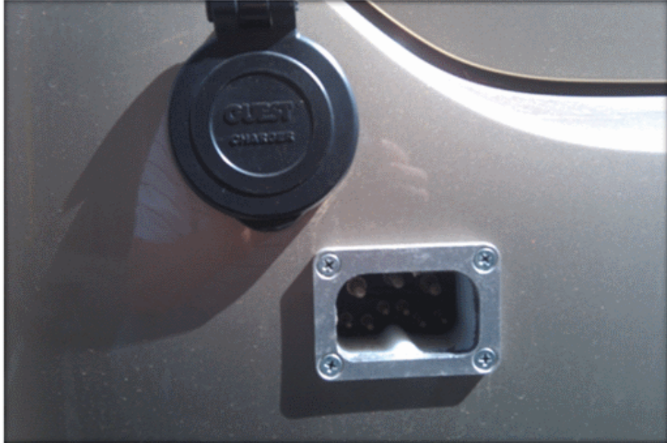
Figure 1. EV100 connector and standard 120-VAC connector that is mounted onto the Prius back bumper.
