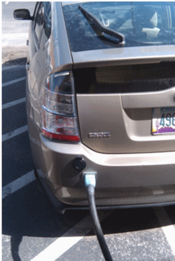
Figure 2. Prius with fast charger connected.
