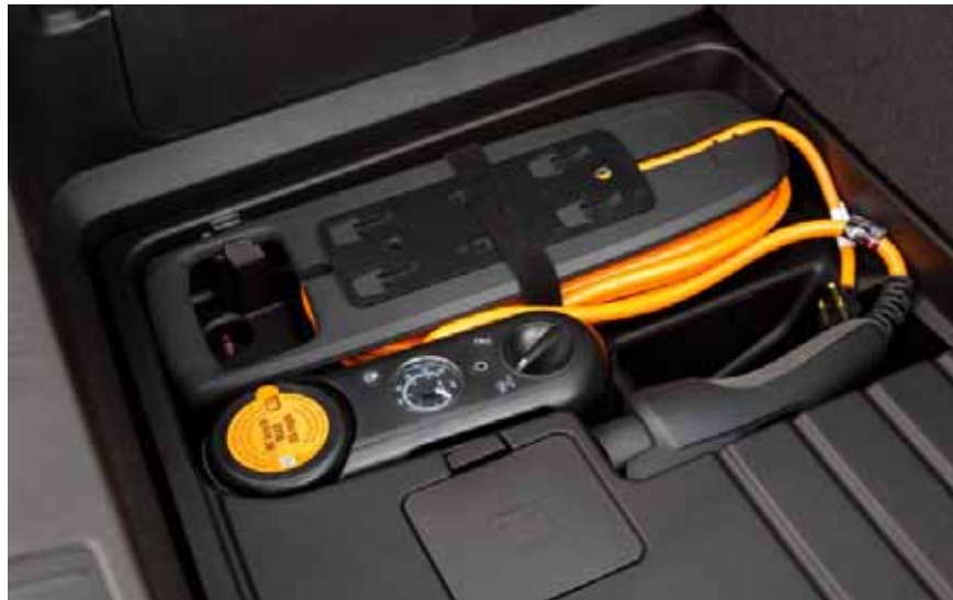
Figure 13. Chevrolet Volt AC Level 1 cordset. 16
