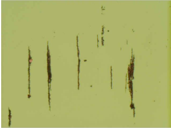
Used oil at 800 hours (100X), bus 73432
