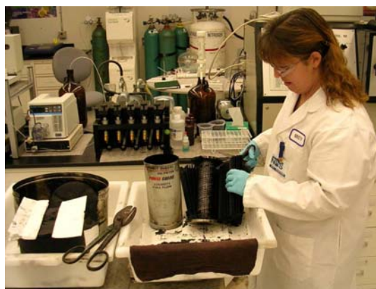
Figure 5. Filter medium being dissected.
