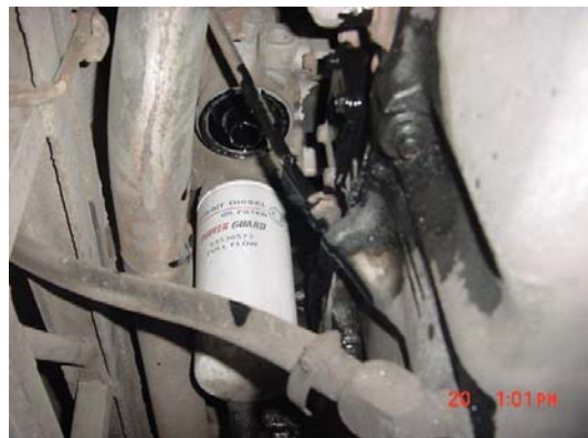
Figure 1. Full-flow filter separated from the engine.
