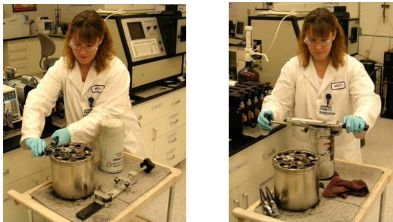
Figure 4. Removing the tops of the bypass filter (left) and full-flow filter (right).
