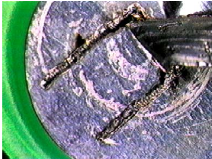
Figure B.8. Aluminum/nickel welds on the positive tab
