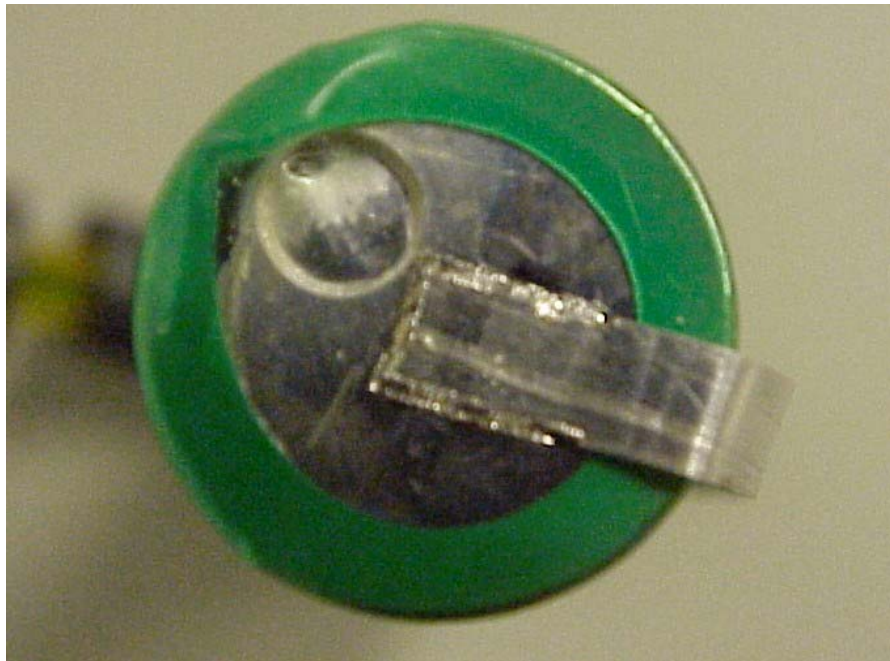
Figure B.7. G2C.60L45.I173.00.NA.NA.L.Q with broken vent and electrolyte leakage.
