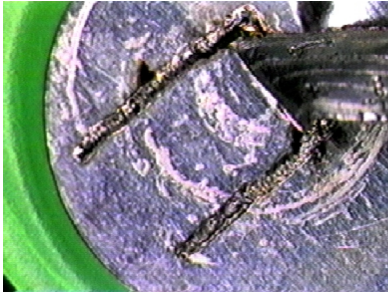
Figure A2.8. Aluminum/nickel welds on the positive tab
