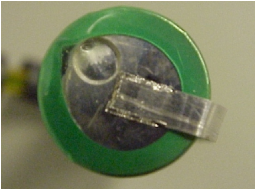
Figure A2.7. G2C.60L45.I173.00.NA.NA.L.Q with broken vent and electrolyte leakage.
