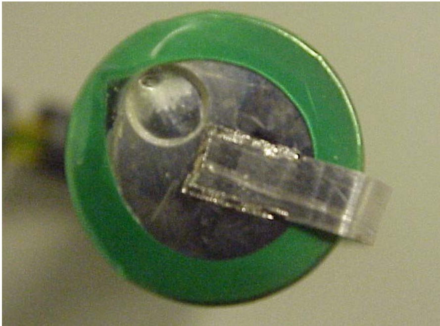
Figure A1.6. G2C.60L45.I173.00.NA.NA.L.Q with broken vent and electrolyte leakage.
