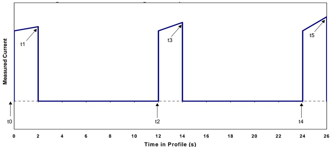
Figure 30. Cold Cranking Resistance Calculation Points
