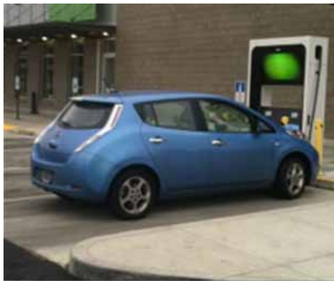
Figure 3-12. Example of an EV Project Nissan Leaf charging at an EV Project DCFC.
