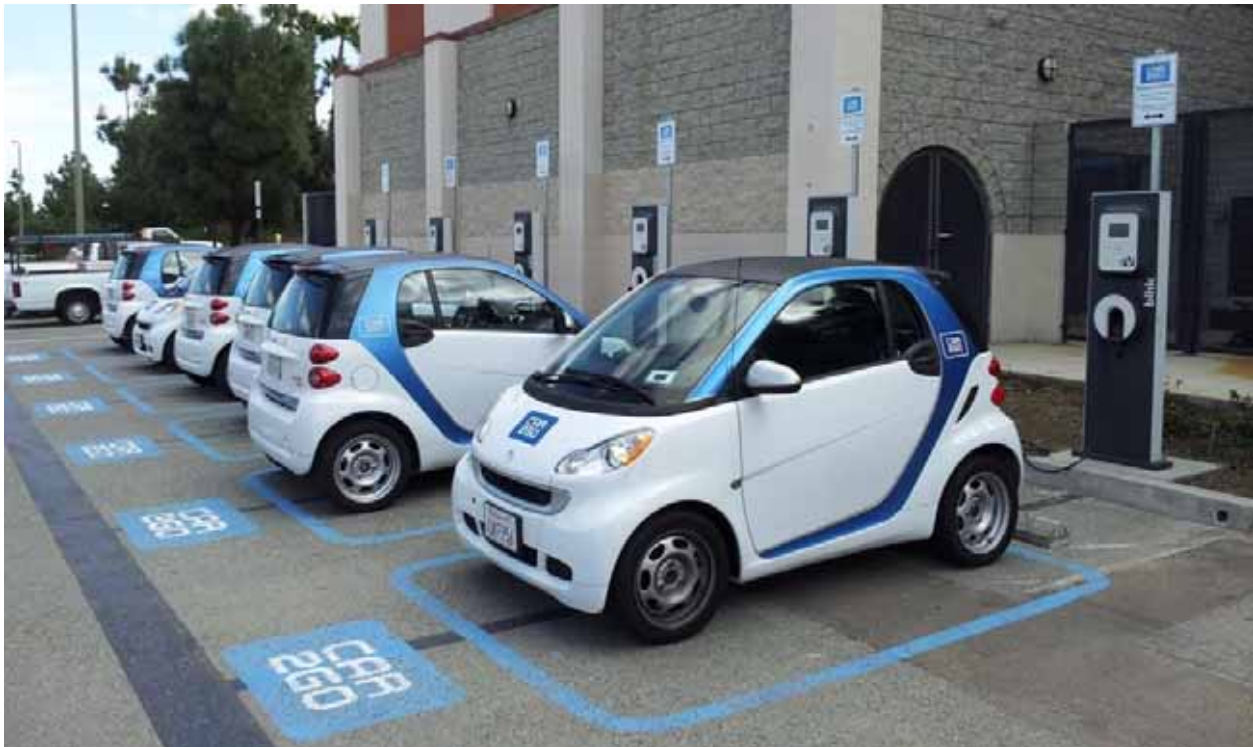
Figure 9-14. Smart Electric Drive Vehicles in the Car2Go fleet parked at an EV Project charging site, with multiple AC Level 2 EVSE, in San Diego.
