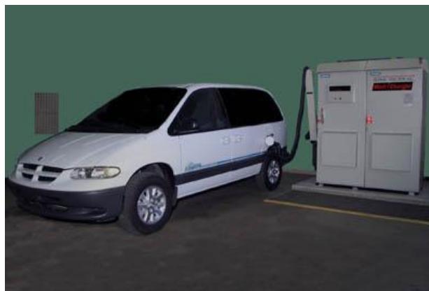
Figure 6-1: Chrysler EPIC DCFC (90kW) circa 1997
