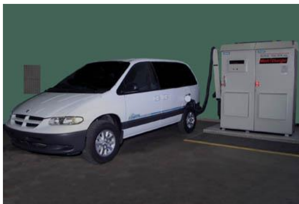
Figure 3-7 Chrysler EPIC DCFC (90kW) circa 1997
