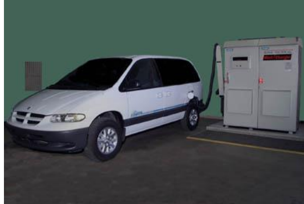
Figure 3-7 Chrysler EPIC DCFC (90kW) circa 1997
