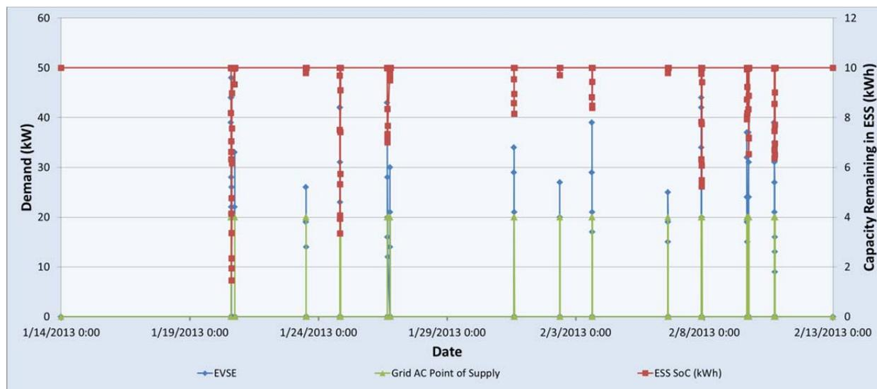
Figure 6 - Simulated power flow for GES-assisted recharging of SDG&E DCFC case study
