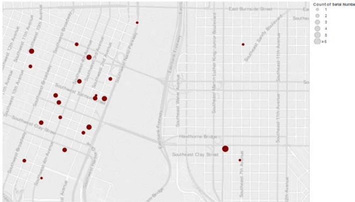
Figure 3. Non-residential AC Level 2 EVSE in Portland, Oregon.
