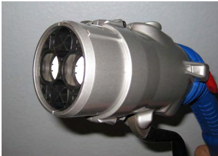
Figure 6. CHAdemo DC Charging Connector
